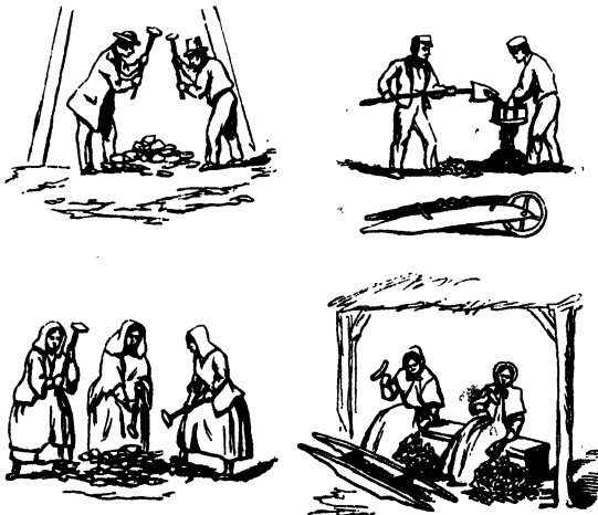
Fig. 166. Ragging, Spalling, Riddling, and Cobbing the Copper Ore.
